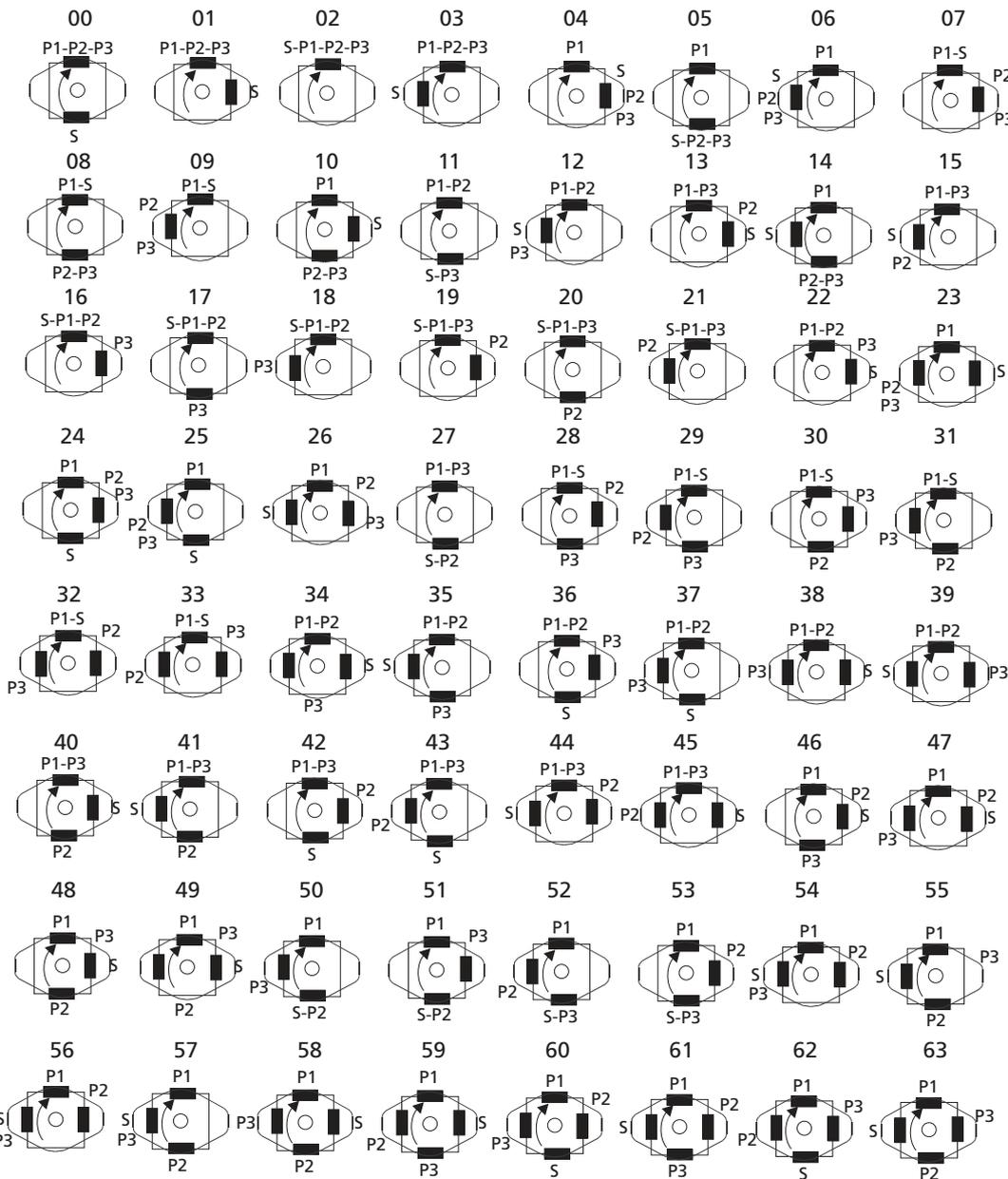
S= Suction port | P1= Shaft end pressure port | P2= Middle pressure port | P3= Cover end pressure port
