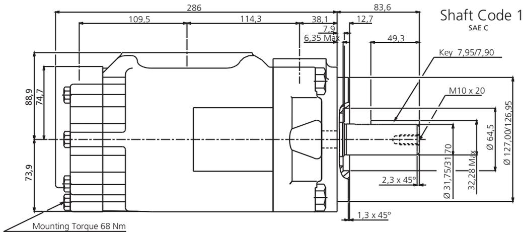
Mounting Torque 68 Nm
