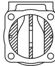
2° - Look at the cartridge to be replaced, if wear is normal just change oil in tank circuit and change or clean filters.
