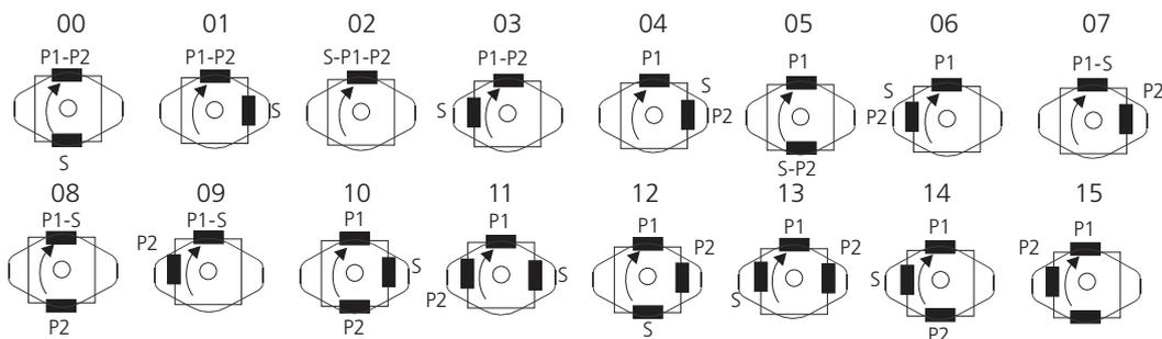
S = Suction port | P1 = Shaft end pressure port | P2 = Cover end pressure port
