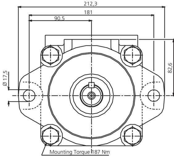
Mounting Torque 187 Nm
