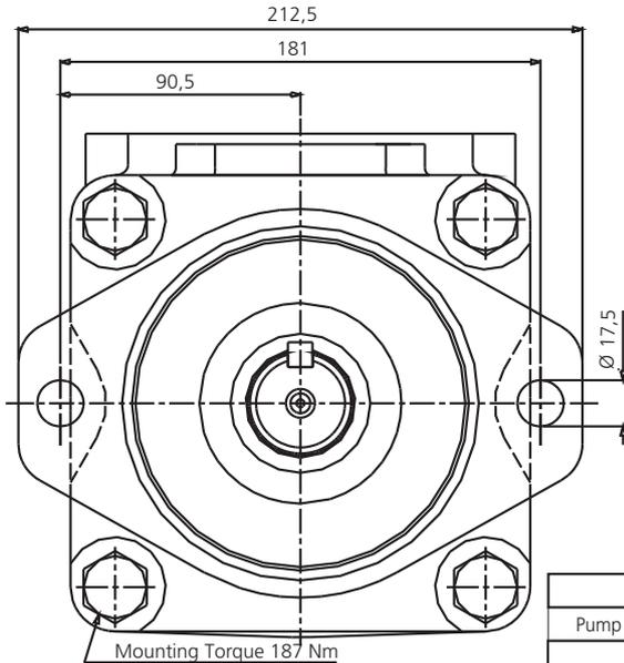
Mounting Torque 187 Nm
