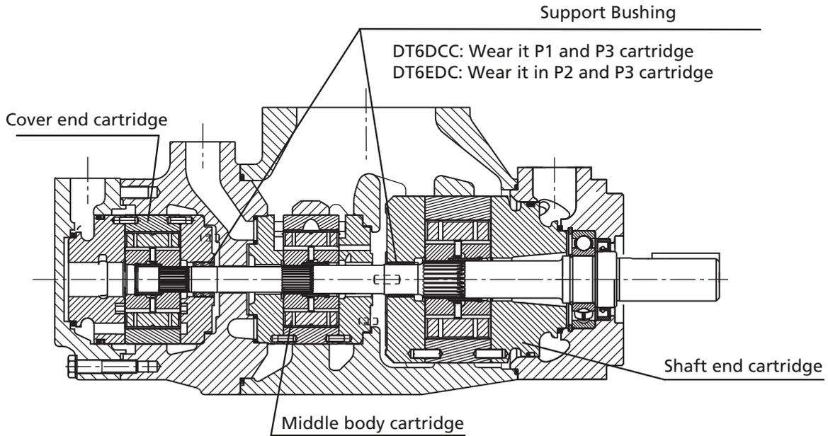
Triple vane pump special feature is that shaft end cartridge is mounted opposite to the middle and cover end kits. Pump, middle cartridge and cover end cartridge rotation always coincide.
