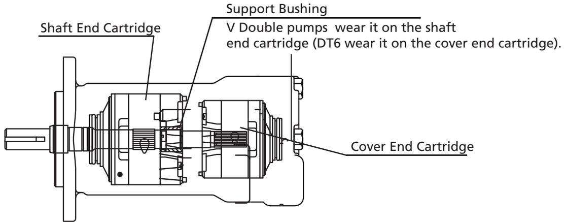
Double pump special feature is that their 2 cartridges are opposite each other, therefore when putting them on the outlet plate, they will apparently have opposite turning sense. Anyway, the arrow in the ring shows the correct rotation. (Pump and cover end cartridge rotation always coincide.)
