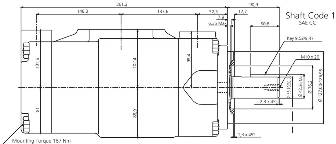
Mounting Torque 187 Nm
